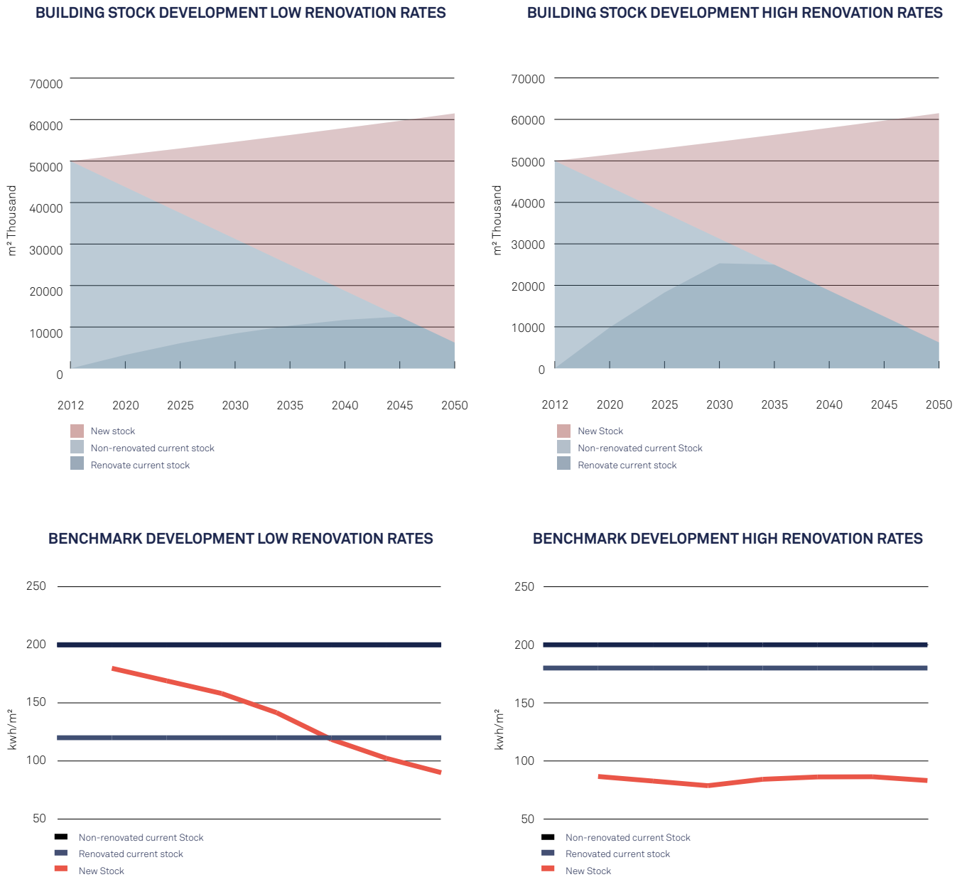
Figure 9: Illustrative calculations of high renovation rates and an ambitious energy standard (left) vs low renovation rates and un-ambitious energy standard (right) on the possible energy level of new buildings to be 2°C-compatible. 12 Both graphs assume the whole building sector achieves 2°C-compatible benchmarks of 93 kWh/m 2 in 2050 and 145 kWh/m 2 in 2030.
